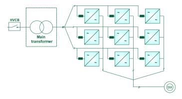
The two AC systems must have different frequencies to limit voltage fluctuations on the individual submodule capacitors. This implies that also the maximum frequency of the SM needs to be below the grid frequency.
