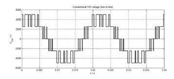
A similar case with a conventional VSI solution (based on 3-level VSI) is also shown. It is obvious, that the THD of the converter voltage is significantly higher.
