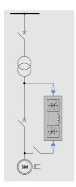
The generator is started via the SFC and once the generator (synchronous machine) is at rated speed and synchronized to the grid the SFC will be bypassed via a bypass switch. The synchronous machine is connected to the grid, the pump-turbine can generate power or consume power from the grid. As the SFC is only used for start-up of the machine, the power rating of the SFC can be lower than the rated power of the machine.
