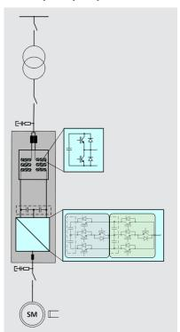
A combination of a modular multilevel converter together with a conventional VSI can reduce the complexity of the converter system.
