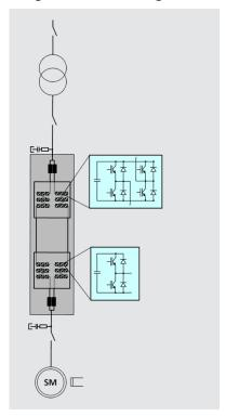
Generally, a conventional VSI can be used. Conventional VSI solutions do not have the restriction of unequal frequencies and thus are suitable for this kind of application. Due to the high harmonic content of the VSI harmonic filter (e.g., sine filter) must be installed on the output and input of the converter.
