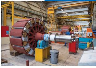
Coil Shop & Stator Winding
